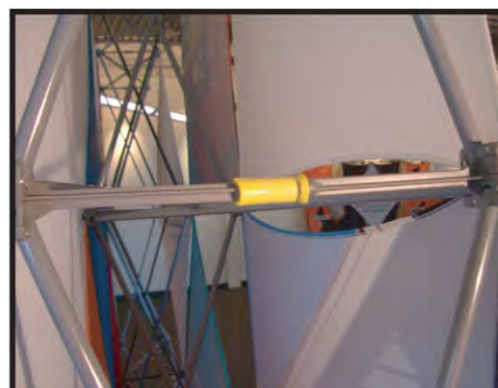
autoXlock may come preinstalled on your display, IMPORTANT make sure to manually release the auto x lock before breaking down.
